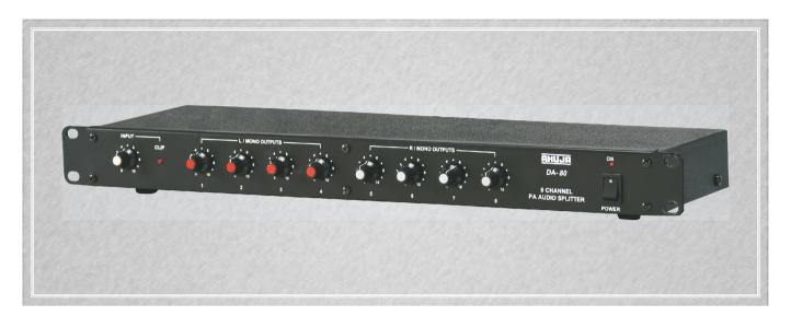
Ahuja introduces a compact and versatile 8 channel audio splitter model DA-80 which splits a mono / stereo line level signal and distributes it to 4 × stereo / 8 × mono line level outputs. This audio splitter effectively overcomes the problem of signal loading which is encountered during cascading of a large number of PA amplifiers / boosters.
